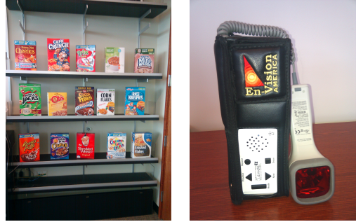
Figure 4. (a) Our mock grocery store shelf stocked with 15 different cereal boxes. (b) The ID Mate II talking barcode scanner from Envision America.
