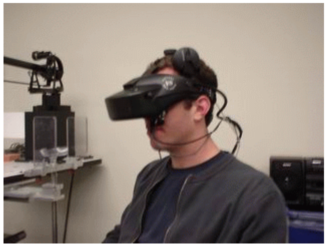
Figure 2: Left: Limbus eye tracker mounted in swim goggle frame. Right: Subject wearing Limbus tracker and HMD with built in video based tracker.
