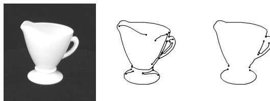
Figure 4: Operation of the recognition system: 1) Image of a cup, 2) boundaries extracted, and 3) curves which keyed matching patches.
