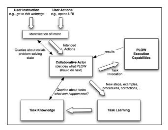
Figure 1: PLOW Architecture
