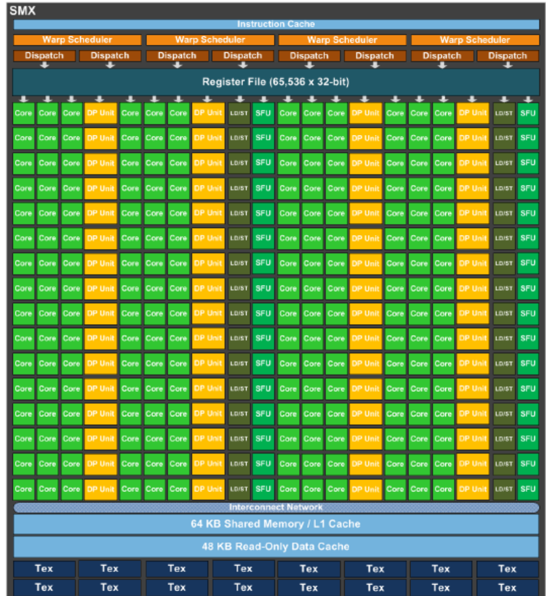
SMX: 192 single-precision CUDA cores, 64 double-precision units, 32 special function units (SFU), and 32 load/store units (LD/ST). Source: Nvidia
