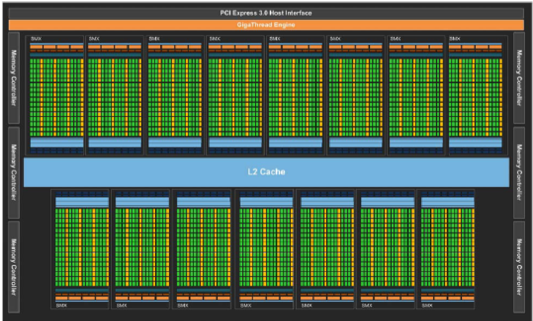
Kepler GK110 Full chip block diagram
