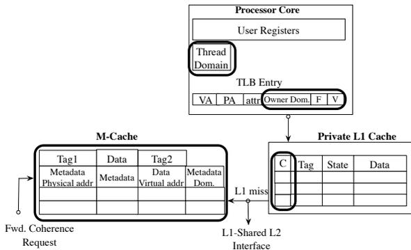
Figure 2: M-cache Mechanism. Dark lines enclose add-ons. Dom.: Domain.
