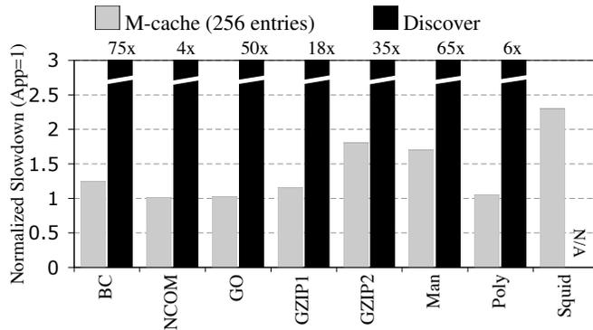
Figure 8: Sentry-Watcher vs. Binary instrumentation. N/A - Discover is not compatible with multi-threaded code. Gzip1 detects Buffer-Overflow bugs. Gzip2 detects memory leak, buffer overflow, and stack smash bugs.
