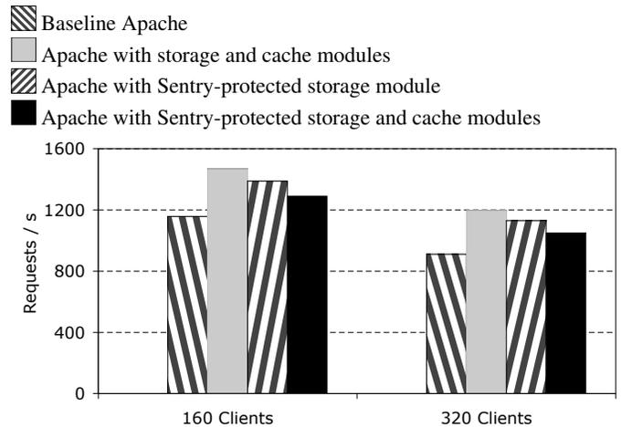
Figure 6: Performance of Sentry-protected Apache with compartmentalized modules.
