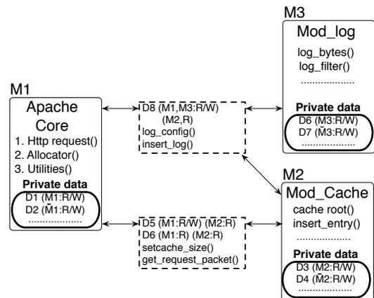
Figure 1: Example of software modules in Apache. M1,M2,M3 — modules, D1...D8 — data elements. Dashed lines indicate data and functions shared between modules. Tuple D: (M:P) indicates module M has permission P on the memory location D. R - Read only ; R/W - Read or Write
