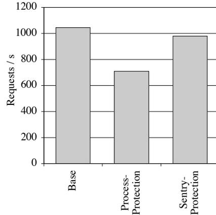
Figure 7: Comparing process-based protection with Sentry. Base: Apache with `mod_case`.
