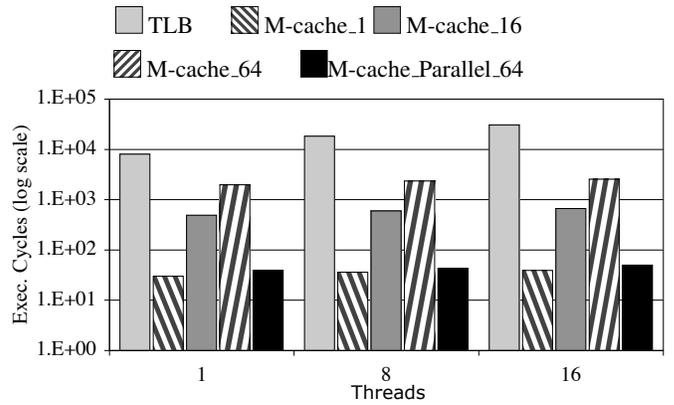
Figure 5: TLB vs. M-cache. M-cache<sub>N</sub> measures execution cycles for changing permissions on N cache lines. L1 handles stores in order. In M-cache\_Parallel\_64, the L1 can sustain 64 concurrent misses.
