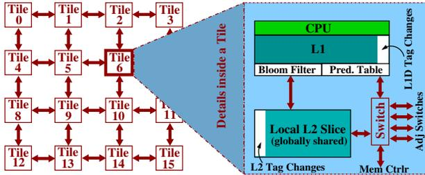
Figure 1. Block diagram of the underlying tiled CMP architecture depicting a processor with 16 cores where the right side highlights details inside a tile with additions for POPS identified by the white (unshaded) regions.
