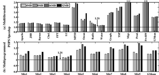
Figure 11. POPS's sensitivity to L2 size for multithreaded and multiprogrammed workloads. For each configuration, POPS performance is normalized to L2S with the correspondingly L2 size.
