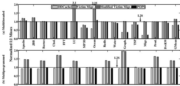
Figure 7. Comparative L2 misses (normalized to L2S) of DDCache, Victim Migration, Modified Victim Migration, and POPS for multithreaded and multiprogrammed workloads.
