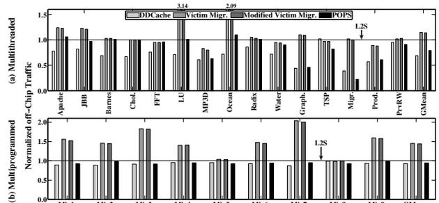
Figure 9. Comparative off-chip traffic generated (normalized to L2S) by DDCache, Victim Migration, Modified Victim Migration, and POPS for multithreaded and multiprogrammed workloads.
