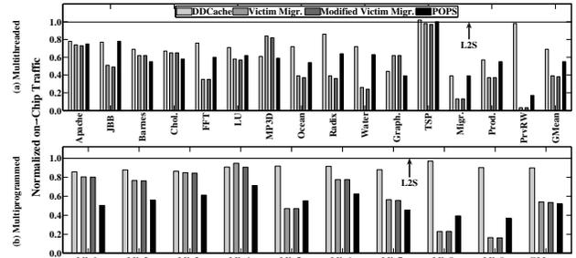
Figure 8. Comparative on-chip traffic generated (normalized to L2S) by DDCache, Victim Migration, Modified Victim Migration, and POPS for multithreaded and multiprogrammed workloads.
