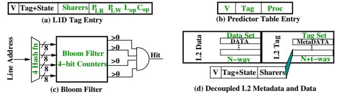
Figure 2. Hardware changes made for POPS. Changes and extra structures are represented using a lighter color.
