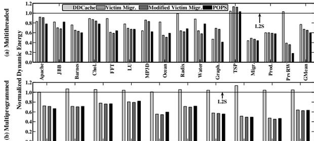
Figure 10. Comparative dynamic energy consumption (normalized to L2S) of DDCache, Victim Migration, Modified Victim Migration, and POPS for multithreaded and multiprogrammed workloads.
