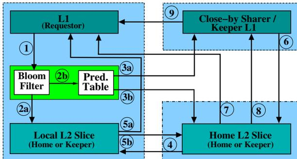
Figure 3. Block diagram showing the flow of messages for a request (L1 miss) among L1 (requestor), bloom filter, predictor table, local L2 slice, close-by L1 (keeper/sharer), and home L2. Shaded regions are used to identify separate tiles. The two shaded regions on the right can be parts of the same (or different) tile.
