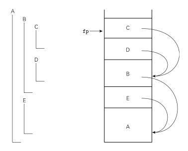
You access a variable in a scope k levels out by following k static links and then using the known offset within the frame thus found.
