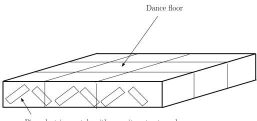
Piezoelectric crystals with capacitors to store charge
