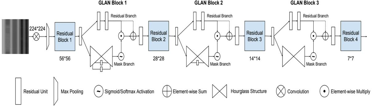
Fig. 4. The structure of the Global Long-sequence Attention Network (GLAN).
