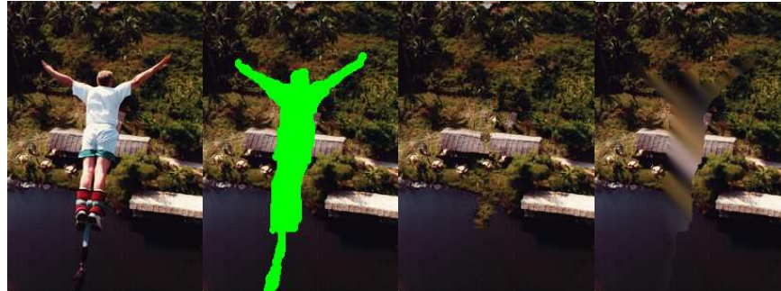
Fig. 6. From left to right: original image (a), inpainting mask (b), exemplar-based result (c), linear interpolation result (d). Pixels selected for inpainting include the bungee jumper and attached rope (shown selected in (b)).
