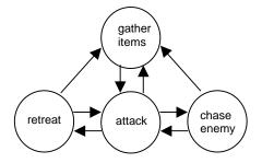
Figure 3.3: Simple FSM for a bot
