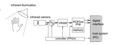
with other sources of illumination, an infrared light source in combination with a specialized infrared-sensitive camera is chosen. Figure 18 shows a system approach, in which the ROFlow-Chip is connected to the infrared-sensitive camera front-end. AD conversion, buffering, and control is introduced to form the interface in between. This way, a field of  $128 \times 128$  image data can be given to the optical flow computation.
