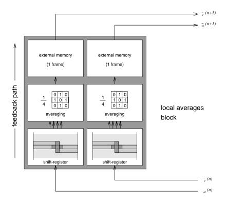
convolution unit, and a one-frame shift register. These components are already known from the description of the preprocessing block and the derivatives block.
