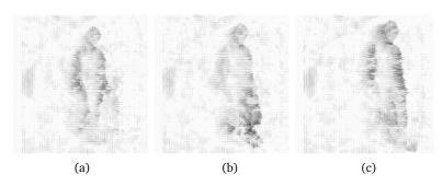
**Figure 15.** Data measured with the sensor translating parallel to a textured wall. The experiment is done with 37.6 frames/s. The values of the x axis are proportional to the camera's speed.
