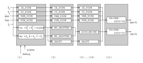
flow components of previous images. At each pixel clock cycle, all inputs must belong to the same pixel location.
