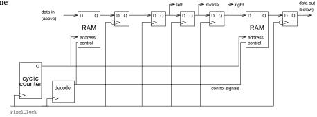
register as a *two-line shift register*. The size of the two-line shift register is dependent on the dimension of the smoothing mask.
