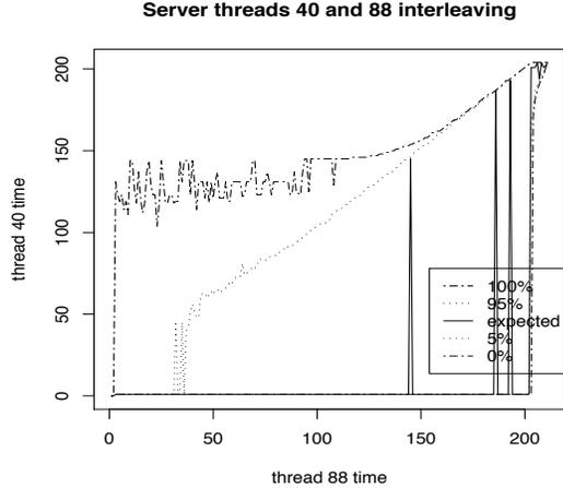
**Figure 2.** The 8-wide histogram of the interleaving between server threads 40 and 88, measured by sampling at rate  $\frac{1}{n}$
