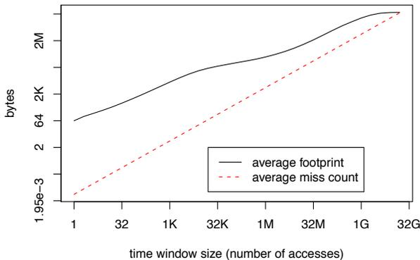
**Figure 5.** Comparison of linear miss count growth and non-linear footprint growth in *Gzip*.
