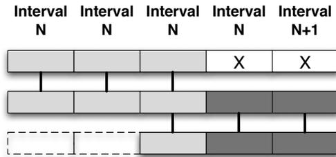
**Figure 6.** Recovery from a permanent fault using FER after BER fails. After interval N fails twice, interval N is re-executed a third time on three processors. Voting identifies the faulty processor, the system rolls back to the beginning of interval N, and execution continues on the remaining two processors.
