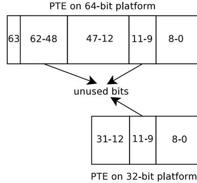
**Figure 2.** Unused bits of page table entry (PTE) for 4K page on 64-bit and 32-bit x86 platforms. Bits 11-9 are hardware defined unused bits for both platforms [IA32-manual, AMD64-manual]. Bits 62-48 on the 64-bit platform are reserved but not used by hardware right now. Our current implementation utilizes 8 bits in this range for maintaining the page hotness counter.
