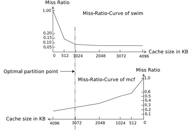
**Figure 5.** An example of our cache partitioning policy between swim and mcf. The cache miss ratio curve for each application is constructed (offline or during an online learning phase) by measuring the miss ratio at a wide range of possible cache partition sizes. Given the estimation of application performance at each cache partitioning point, we determine that the best partition point for the two applications is if 1 MB cache is allocated to swim and 3 MB cache to mcf.
