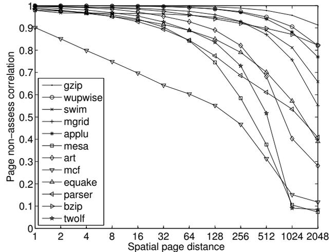
**Figure 3.** Illustration of page non-access correlation as a function of the spatial page distance. Results are for 12 SPEC CPU2000 benchmarks with 2-millisecond sampled access time windows. For each distance value  $D$ , the non-access correlation is defined as the probability that the next  $D$  pages are not accessed in a time window if the current page is not accessed. We take snapshots of each benchmark’s page table every 5 seconds and present average non-access correlation results here.
