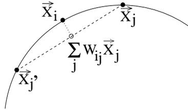
Figure 3: A data point  $\vec{X}_i$ , its neighbors  $\vec{X}_j$ , and its locally linear reconstruction  $\sum_j W_{ij} \vec{X}_j$ . The reconstruction weights are constrained to satisfy  $\sum_j W_{ij} = 1$ .
