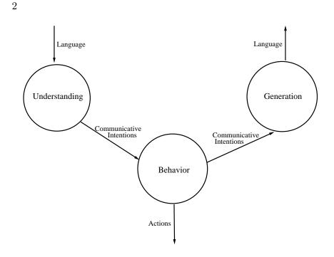
Figure 1.1. Conceptual Subsystems of a Conversational Agent
