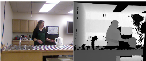
Figure 3: Kinect data frame showing RGB and depth streams.
