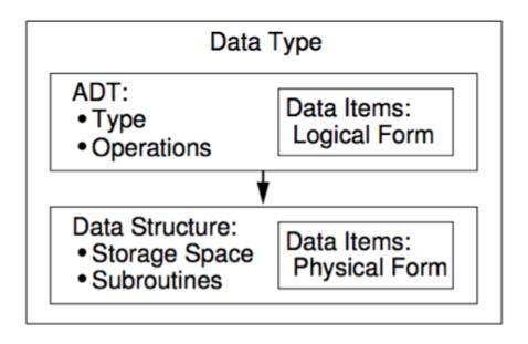
The relationship between data items, abstract data types, and data structures. The ADT defines the logical form of the data type. The data structure implements the physical form of the data type.
