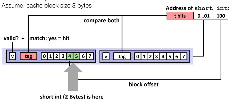
E = 2: Two lines per set Assume: cache block size 8 bytes Address of short int: 0...01 t bits 100 compare both match: yes = hit valid? + 0 1 2 3 4 5 6 7 tag block offset short int (2 Bytes) is here
