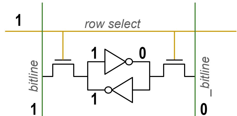
**Note: The two access transistors should be NMOS, rather than PMOS. Corrected after the class.**
