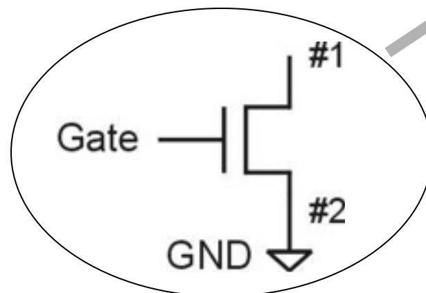
Terminal #2 must be connected to GND (0V).
