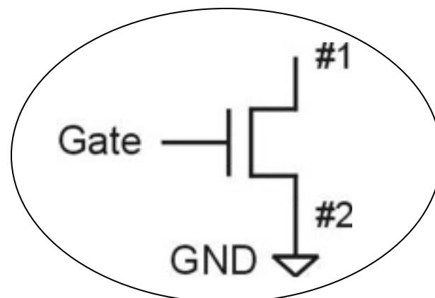
Terminal #2 must be connected to GND (0V).
