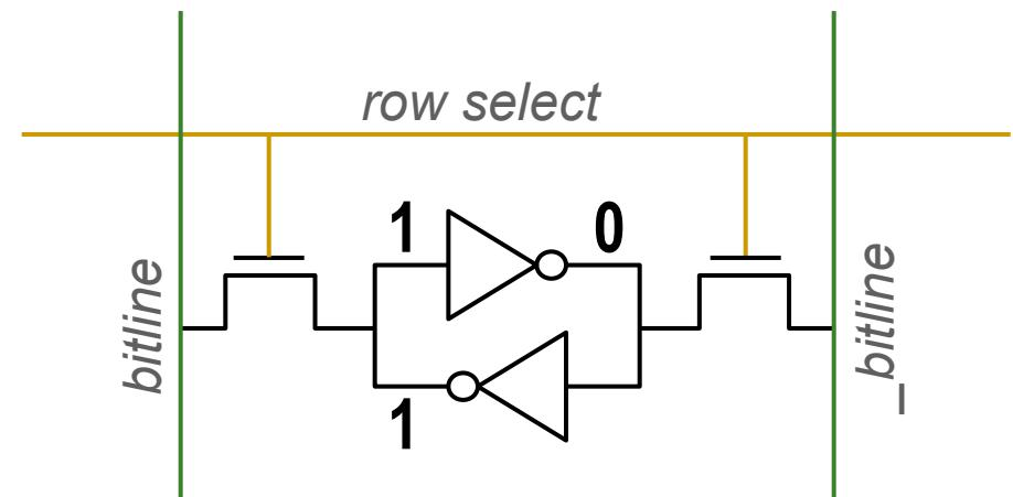
**Note: The two access transistors should be NMOS, rather than PMOS.
