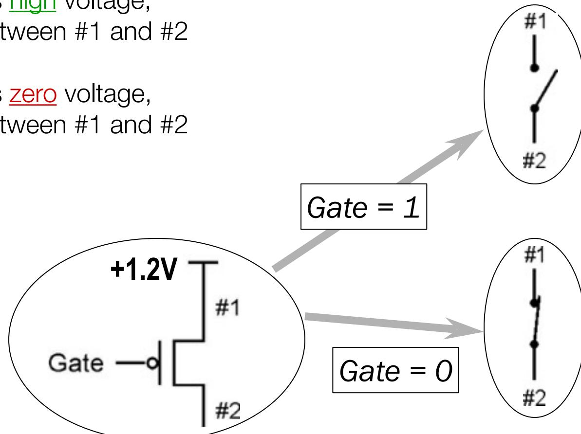
Terminal #1 must be connected to +1.2V
