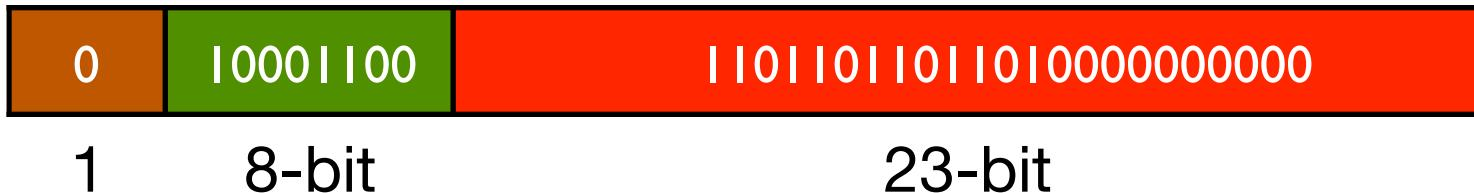
$$\begin{aligned} 15213_{10} &= 11101101101101_2 \\ &= (-1)^0 1.\underline{1101101101101}_2 \times 2^{13} \end{aligned}$$
