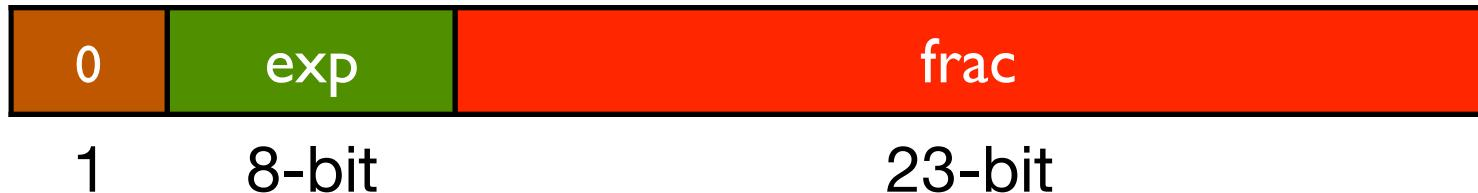
$$\begin{aligned} 15213_{10} &= 11101101101101_2 \\ &= (-1)^0 1.1101101101101_2 \times 2^{13} \end{aligned}$$
