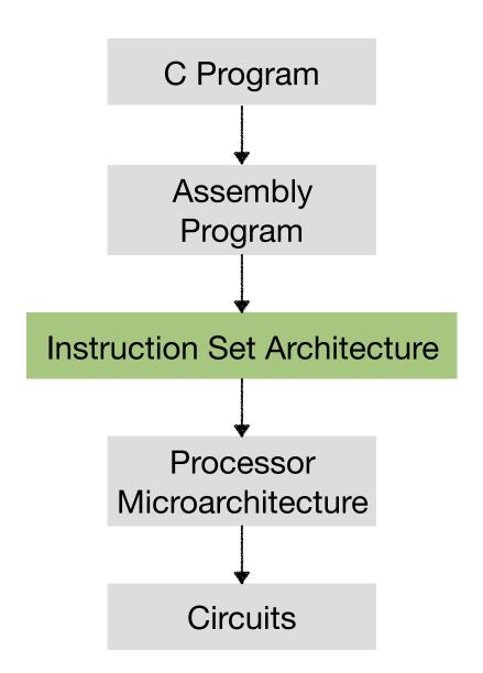
ISA is the interface between assembly programs and microarchitecture
