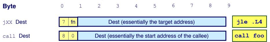
• The instruction length limits how far you can jump/call functions. What if the jump target has a very long address that can't fit in 8 bytes?
