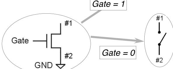
Terminal #2 must be connected to GND (0V).
