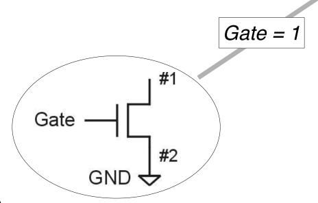
Terminal #2 must be connected to GND (0V).
