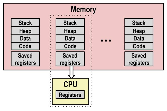
• Load saved registers and switch address space (context switch)
