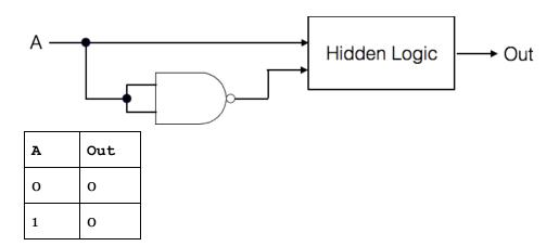
(3 points) What is the functionality of the hidden logic in the circuit? You can denote the two inputs to the hidden logic as In1 and In2.
