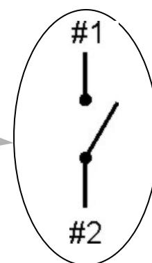
Terminal #2 must be connected to GND (0V).
