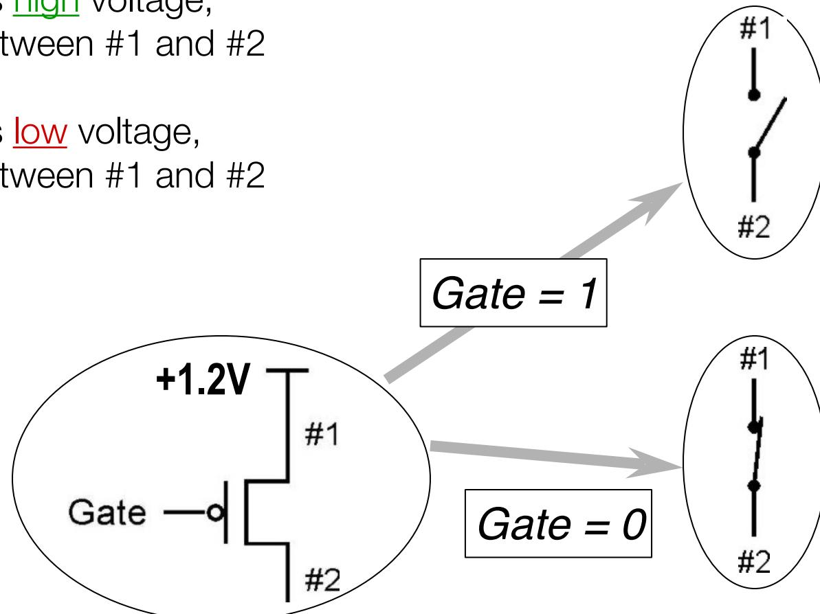
Terminal #1 must be connected to +1.2V
