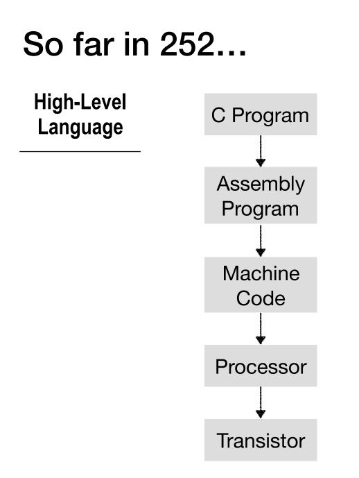
**High-Level** C Program Language Assembly Program **Instruction Set Architecture** (ISA) Machine Code Processor Transistor
