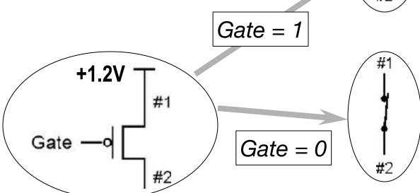
Terminal #1 must be connected to +1.2V
