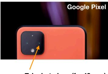
Telephoto lens (f = 48 mm) + computational photography algorithm for super resolution
