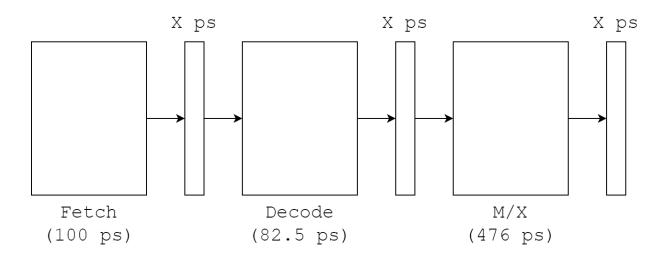
The three stages take 100 ps, 82.5 ps, and 476 ps, respectively. The fastest clock frequency this pipeline is capable of is 2.0 GHz. How long must it take to latch data into each of the 3 intermediate pipeline registers? Answer in picoseconds. A picosecond (ps) is 10<sup>-12</sup> second.
