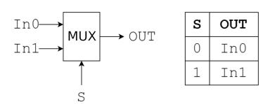
We can construct other basic logic gates using only MUXes. For instance, we can construct a 2-input OR gate that computes **A** OR **B** using a two-input MUX by setting its inputs as follows:
