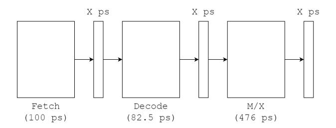
The three stages take 100 ps, 82.5 ps, and 476 ps, respectively. The fastest clock frequency this pipeline is capable of is 2.0 GHz. How long must it take to latch data into each of the 3 intermediate pipeline registers? Answer in picoseconds. A picosecond (ps) is  $10^{-12}$  second.
