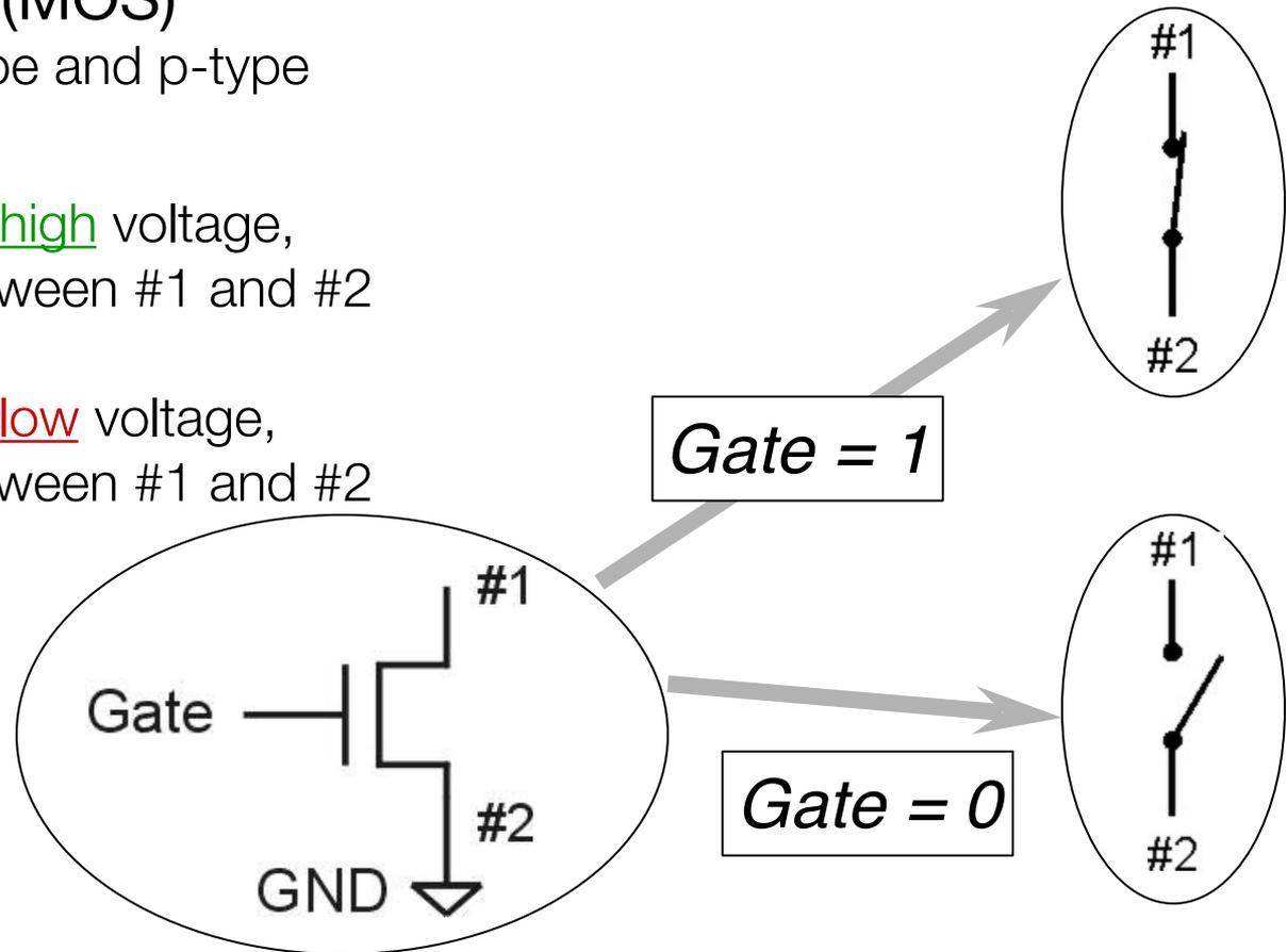
Terminal #2 must be connected to GND (0V).
