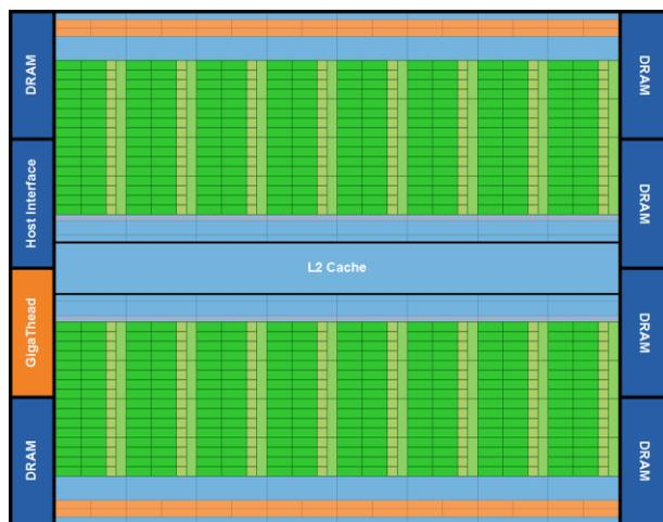
Fig. 1. Architecture of NVidia Fermi GPU
