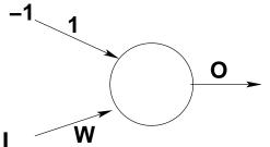
Here is a one-input perceptron with its threshold  $\theta$  implemented as a constant -1 input multiplied by a constant weight (here set to 1). The input *I* (that's not a "one") is weighted by *W*, and initially W = 1. Its output is labeled *O* (that's not a "zero").
