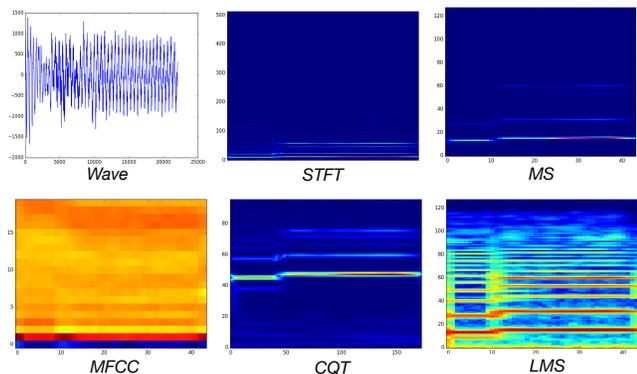
**Figure 3: Different representations of audio that are fed to the sound encoder network. The horizontal axis is time and the vertical axis is amplitude (for Wave), frequency (for STFT, MS, CQT, and LMS) or quefrency (for MFCC).**
