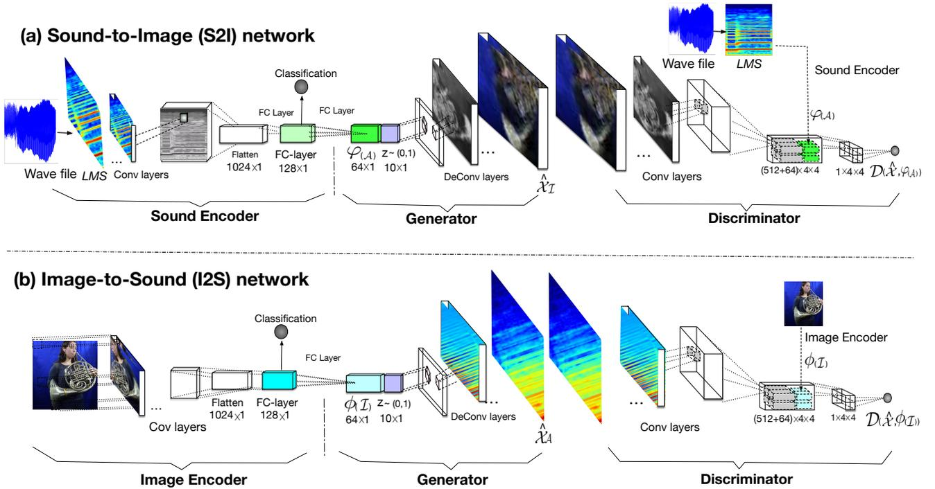
Figure 2: The overall diagram of our model. This figure consists of (a) an S2I GAN network and (b) an I2S GAN network. Each network contains an encoder, a generator and a discriminator, respectively.
