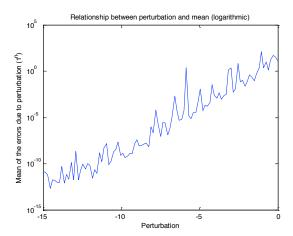
As can be seen in this graph, as the perturbation decreases so does the mean of the errors, the mean of the errors approaches 0 suggesting that the error due to perturbation decreases. Note that the logarithmic scale shows a somewhat linear decrease (because the scale is logarithmic). Note that the spikes occur due to anomalies in the data as the matrices are generated at random, despite this the data still follows a sure path.
