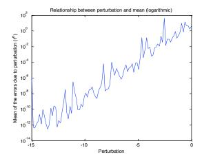
As can be seen in this graph, as the perturbation decreases so does the mean of the errors, the mean of the errors approaches 0 suggesting that the error due to perturbation decreases. Note that the logarithmic scale shows a somewhat linear decrease (because the scale is logarithmic). Note that the spikes occur due to anomalies in the data as the matrices are generated at random, despite this the data still follows a sure path.
