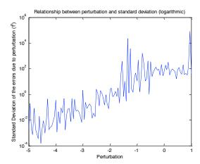
Similarly, while the standard deviation of the system also portrays an exponential relationship, the error due to perturbation is much larger in the ill conditioned system. This is different from the regular systems because here the error is in the magnitude of 10 -2 whereas before it was 10 -4. This shows that the ill system has caused the system to be harder to solve.
