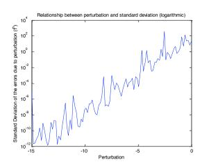
Similarly, this graph shows that the standard deviation of the errors also falls as the perturbation falls. The standard deviation approaches 0 because all the values of error are more condensed and approach zero. Note that the logarithmic scale shows a somewhat linear decrease (because the scale is logarithmic).
