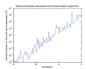
Similarly, this graph shows that the standard deviation of the errors also falls as the perturbation falls. The standard deviation approaches 0 because all the values of error are more condensed and approach zero. Note that the logarithmic scale shows a somewhat linear decrease (because the scale is logarithmic).
