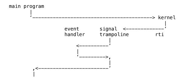
Note that because the main program and signal handler run on the same thread, they can't use scheduler-based locks to synchronize access to shared data structures. Rather (as we saw in the implementation of thread scheduling in Chap. 13), the main program needs to turn off signals while manipulating data that may also be accessed in a handler.
