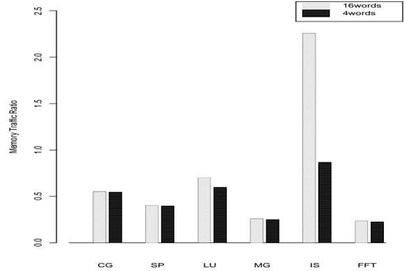
Figure 10: Traffic ratio for 16 and 4 word lines on a 1Mw cache
