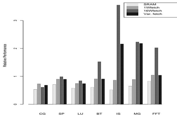
Figure 11: Normalized execution time under different fetching policies for a 64Kw cache
