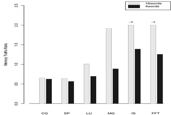
Figure 9: Traffic ratio for 16 and 4 word lines on a 64Kw cache
