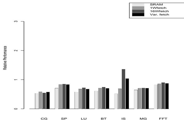
Figure 12: Normalized execution time under different fetching policies for a 1Mw cache
