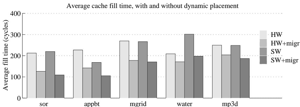
Figure 3: Average fill time, for 64 processors and 64-byte cache blocks.
