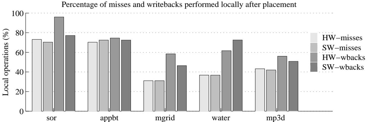
Figure 2: Local cache activity, for 64 processors and 64-byte cache blocks.
