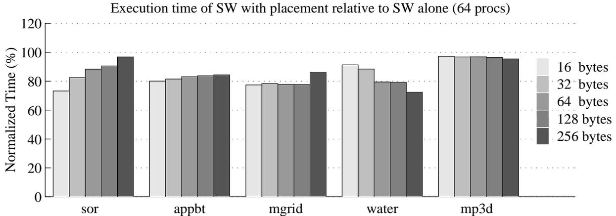
Figure 5: Normalized execution times for varying block sizes under software coherence.
