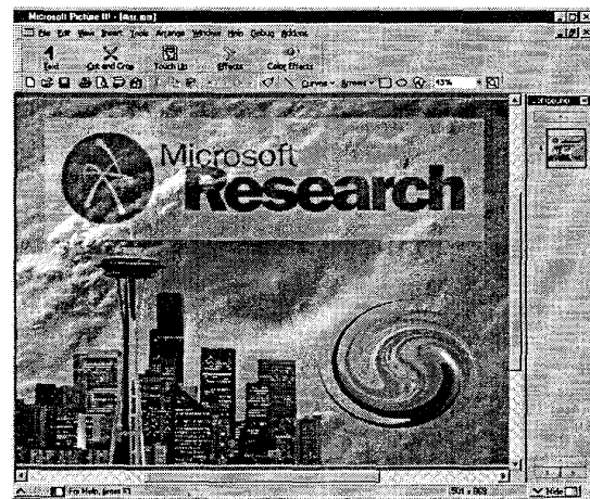
Fig. 2. Executing a Profiling Scenario. With Coign instrumentation in place, the application is run through one or more profiling scenarios to measure inter-component communication. In this scenario, Picture It! loads and renders a composite image.
