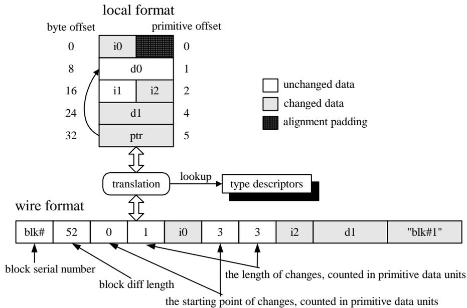
Figure 4: Wire format translation of a structure consisting of three integers (`i0`–`i2`), two doubles (`d0`–`d1`), and a pointer (`ptr`). All fields except `d0` and `i1` are changed.
