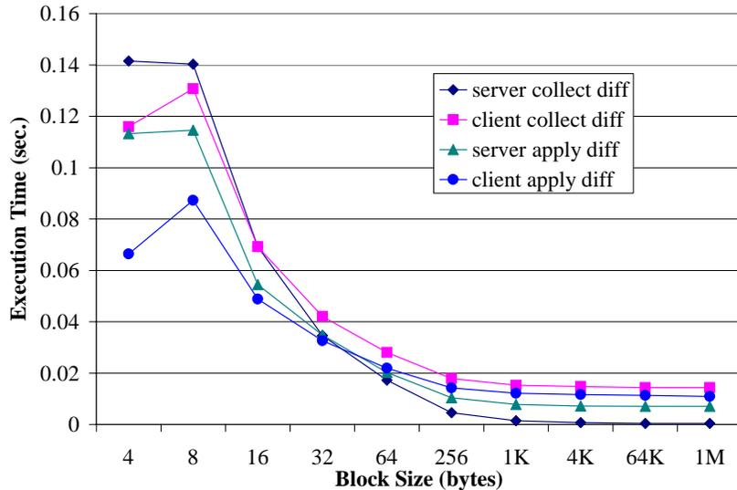
Figure 11: The effect of varying block size.
