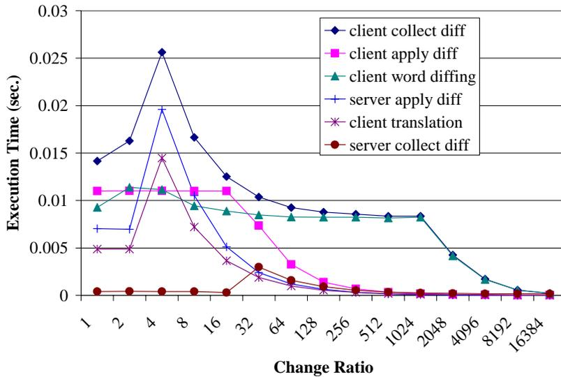
Figure 10: Diff management cost as a function of modification granularity (1MB total data).
