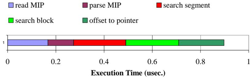
Figure 9: Breakdown of swizzling MIPs into local pointers (using `cross 1024`).
