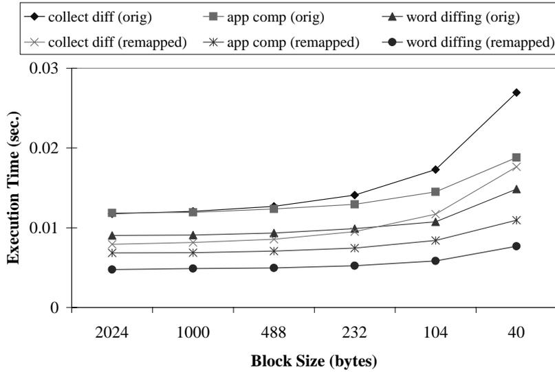
Figure 12: Performance impact of version based block layout, with 1MB total data.
