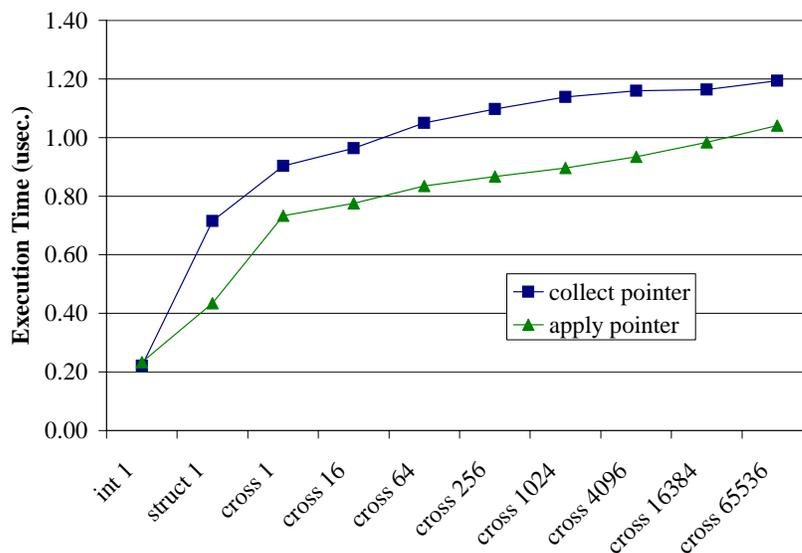
Figure 7: Pointer swizzling cost as a function of pointed-to object type.
