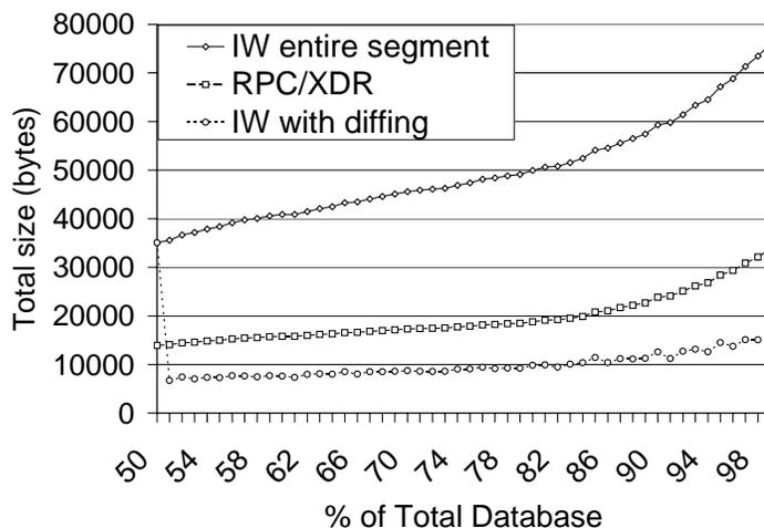
Figure 16: Wire format length of datamining segment under InterWeave and RPC.
