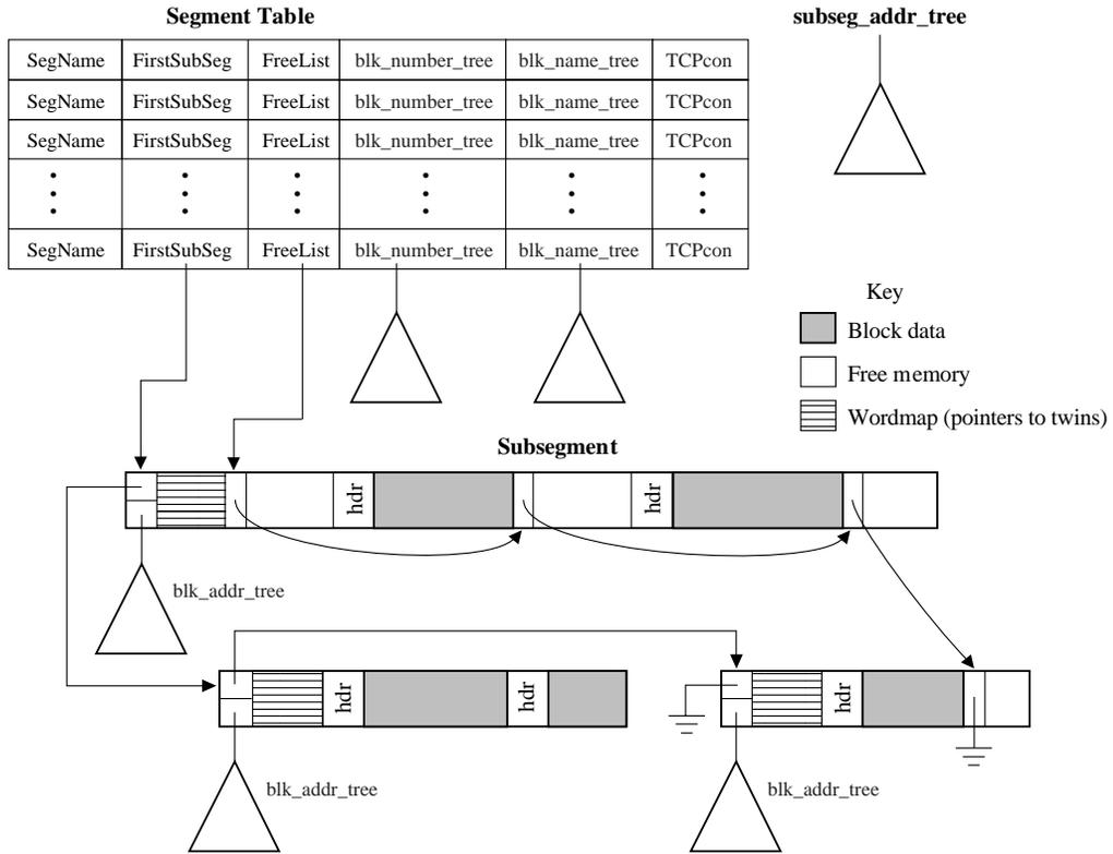
Figure 2: Simplified view of InterWeave client-side data structures: the segment table, subsegments, and blocks within segments. Type descriptors, pointers from balanced trees to blocks and subsegments, and footers of blocks and free space are not shown.
