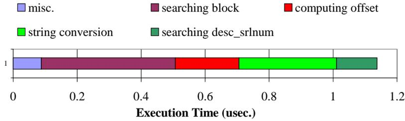
Figure 8: Breakdown of swizzling local pointers into MIPs (using `cross 1024`).
