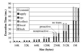
Figure 1. Execution time for transactions that transmit a large amount of data on a LAN.
