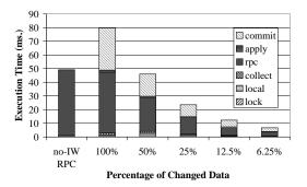
Figure 3. Execution time for "proactive transaction" running on a LAN, when both the caller and callee only update x% of a 1MB segment.
