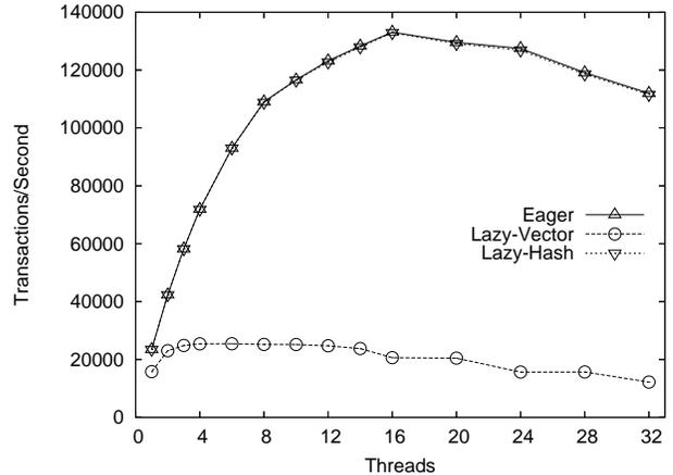
**Figure 1.** Workload with large write sets, modeled as a linked list with 8-bit keys, 95% lookups, and 5% overwrites. The list is pre-populated to store all elements in the range 0–255. Overwrite transactions modify every node in a randomly selected list prefix. Adding a hash table for fast write set lookups eliminates the performance gap between eager and lazy acquisition.
