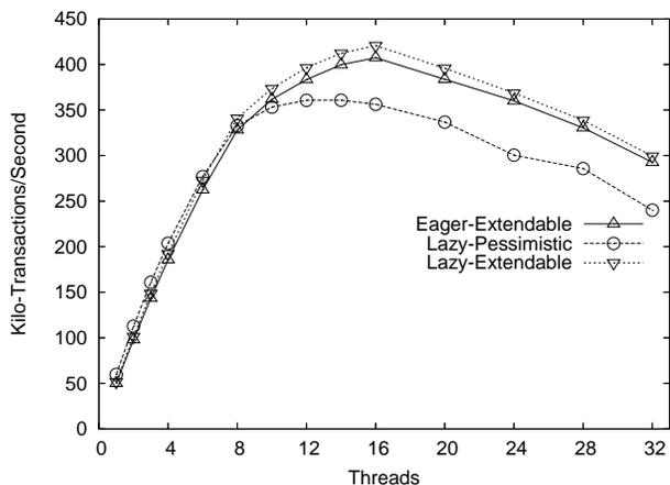
**Figure 2.** Linked List with 8-bit keys, and an 80/10/10 lookup, insert, remove ratio (no overwrites). The list is pre-populated to store half of the elements in the range 0–255. TL2-style timestamps (pessimistic) scale noticeably worse than the “extendable” timestamps of Riegel et al. With extendable timestamps, eager and lazy acquire are almost indistinguishable.
