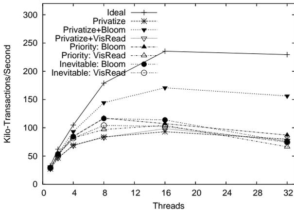
**Figure 7.** Extensible Hashing. Each transaction performs 8 random puts into an extensible hash table. Rehashing can be performed inevitably, with priority, or via privatization (locking). Ideal uses a large table that never requires rehashing for this workload.
