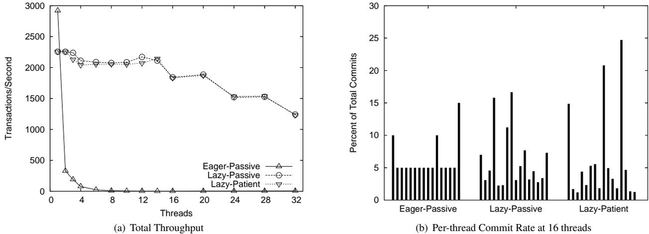
**Figure 4.** Pathological microbenchmark. All threads transactionally access a 1024-element doubly-linked list, reading every entry and modifying 8 entries. There are no write-write conflicts, but with half of the threads forward-traversing and half the threads traversing in reverse, eager acquire is prone to livelock. Note that in the graph at right, eager-passive threads are getting relatively fair slices of an almost nonexistent pie.
