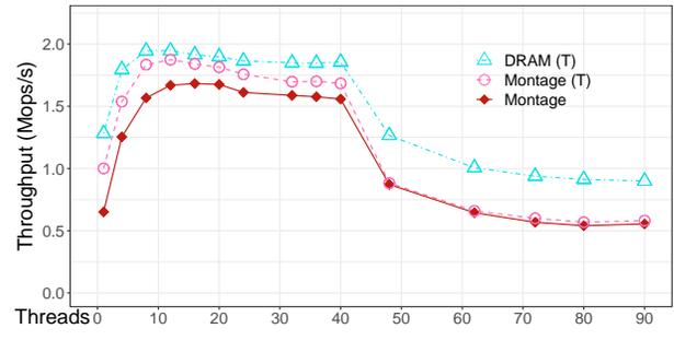
Figure 10: memcached throughput on YCSB-A (linear  $y$ -axis).
