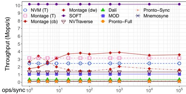
Figure 9: Throughput of 40-thread hashmaps with a sync every  $x$  operations on average (log-scale  $x$ -axis; linear  $y$ -axis).
