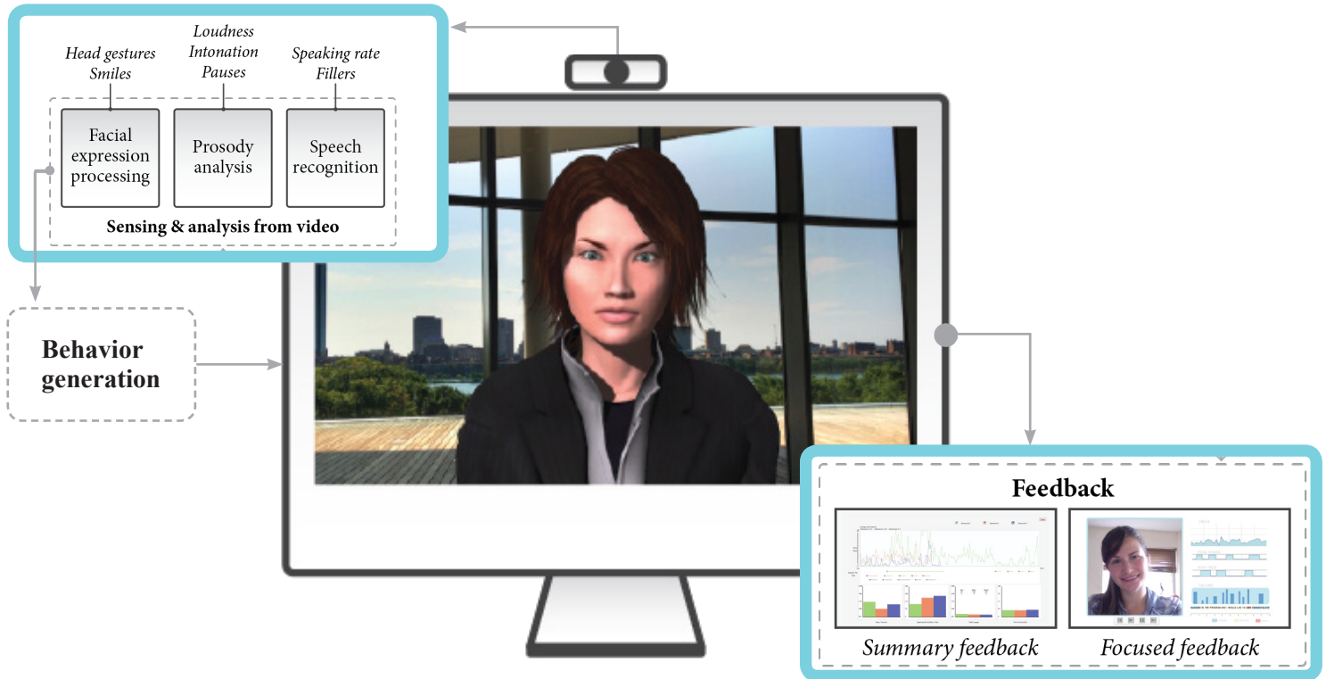
Figure 1: The MACH system works on a regular laptop, which processes the audio and video inputs in real time. The data is used to generate the behavior of a three-dimensional character that interacts with participants and provides feedback.
