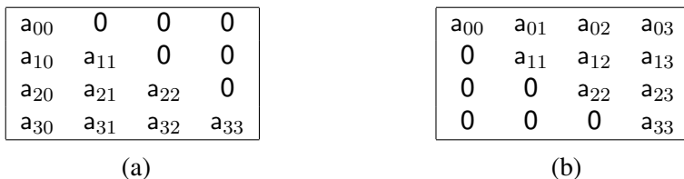
Figure 12.6 Triangular matrices. (a) A lower triangular matrix. (b) An upper triangular matrix.
