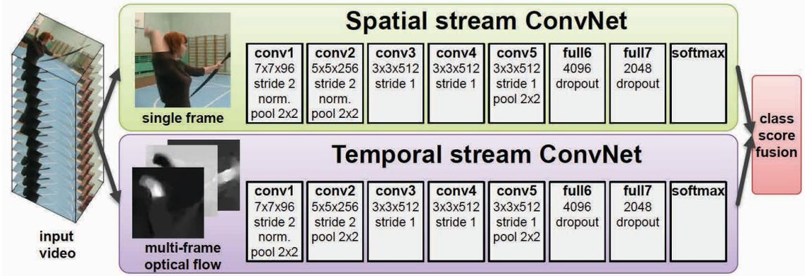
Figure 2.4: An overview of the two-stream ConvNet architecture. Figure from [175].
