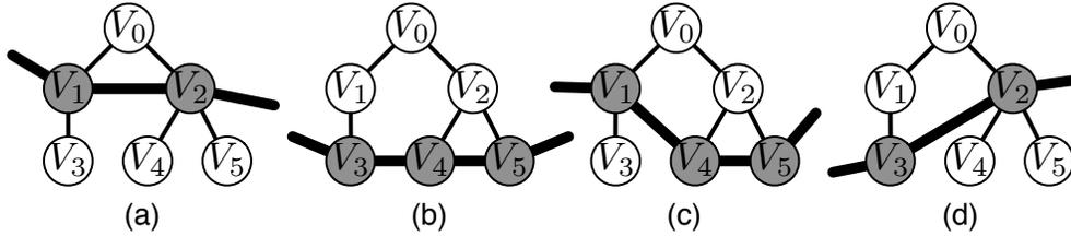
Figure 6.4: Slices in the example supervoxel tree. (a) - (d) list all 4 possible slices of the segmentation tree (excluding the root node). Each slice is highlighted as a thick black curve, and nodes on the slice are darkened.
