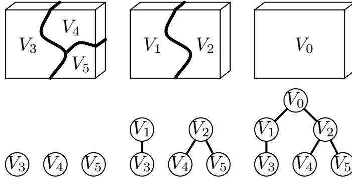
Figure 6.3: Illustration of the segmentation tree creation process. On the top of the figure, left, middle and right are bottom-up levels in a supervoxel hierarchy:  $T^1$ ,  $T^2$  and  $T^3$  respectively. From left to middle,  $V_4$  and  $V_5$  are merged together, and  $V_3$  remains itself as  $V_1$  in the middle. From middle to right,  $V_1$  and  $V_2$  are merged together to a single top node  $V_0$ . The corresponding tree-graphs are in the bottom row.
