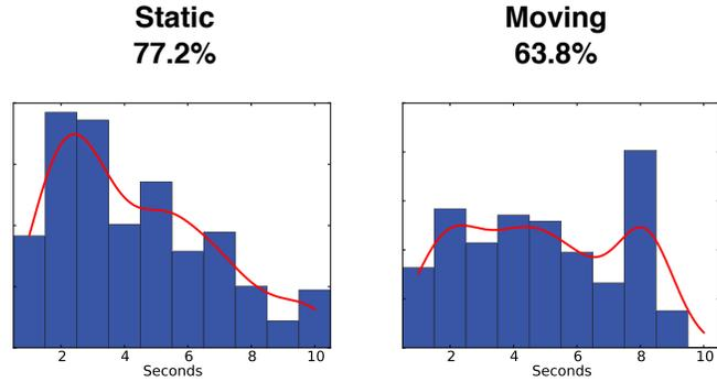
Figure 5.7: Performance comparison between static background and moving background. The percentages on top are computed when both the actor and action of supervoxel perception are correctly matched to ground truth. The response time plots include both correctly and incorrectly matched supervoxel perceptions.
