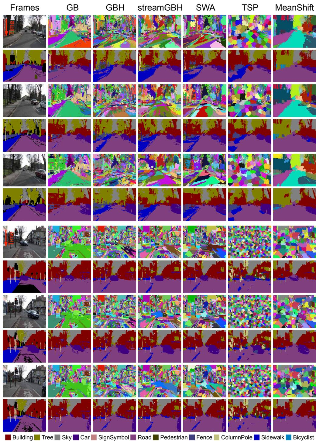
Figure 3.9: Example results on two short clips from the CamVid daytime test video. Images in the first column are video frames and groundtruth labels and the remaining columns are individual methods with supervoxel segmentation and semantic labeling on supervoxels.
