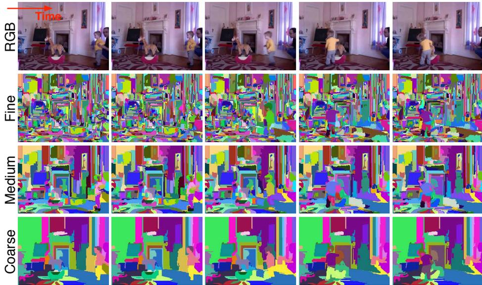
Figure 5.1: Example output of the streaming hierarchical supervoxel method in Chapter IV. From left to right columns are frames uniformly sampled from a video. From top to bottom rows are: the original RGB video, the fine segmentation (low level in the hierarchy), the medium segmentation (middle level in the hierarchy), and the coarse segmentation (high level in the hierarchy).
