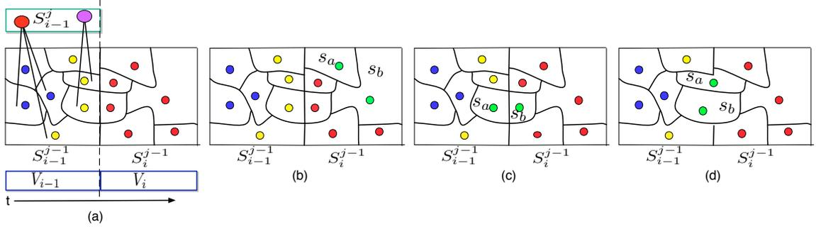
Figure 4.5: Example of the three cases in the additional merging criteria: (a), the initial status of semi-supervised grouping; (b-d) three different cases, when  $s_a$  and  $s_b$  needed to be merged: (b)  $s_a \subset S_i^{j-1}$  and  $s_b \subset S_i^{j-1}$ ; (c)  $s_a \cap S_{i-1}^{j-1} \neq \emptyset$  and  $s_b \subset S_i^{j-1}$ ; (d)  $s_a \cap S_{i-1}^{j-1} \neq \emptyset$  and  $s_b \cap S_{i-1}^{j-1} \neq \emptyset$
