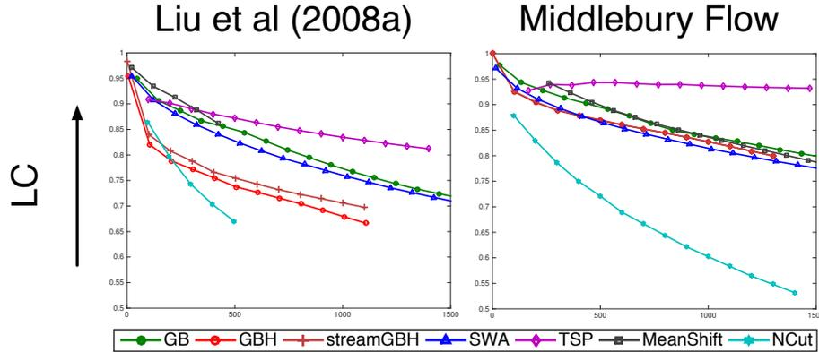
Figure 3.5: Plots for Label Consistency (LC) based on the number of supervoxels **per-frame** (x-axis). Black arrow indicates the direction of better performance. Plotted dots are the average score of linear-interpolated values from all videos in a dataset at the same number of supervoxels per-frame.
