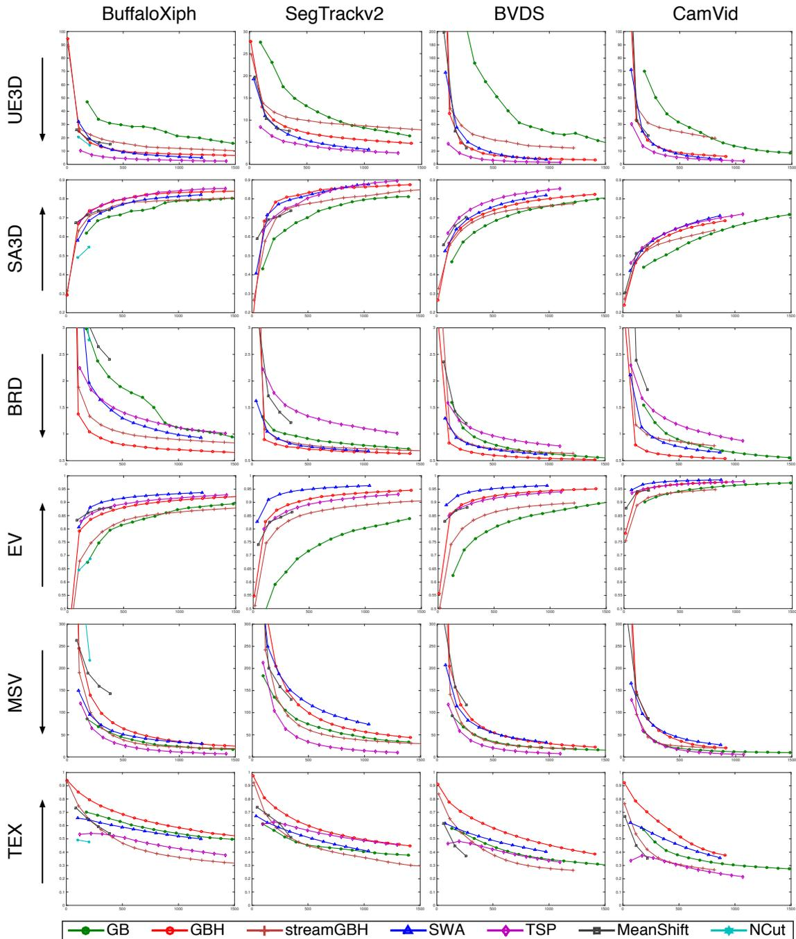
Figure 3.3: Graphs plot the number of supervoxels **per-frame** (x-axis) against various metrics (y-axis). Datasets are organized by columns and metrics are organized by rows. Black arrows in each row are used to indicate the direction of better performance with regard to the metric. Plot ranges along the y-axis are aligned for all metrics except UE3D. Plotted dots are the average score of linear-interpolated values from all videos in a dataset at the same number of supervoxels per-frame.
