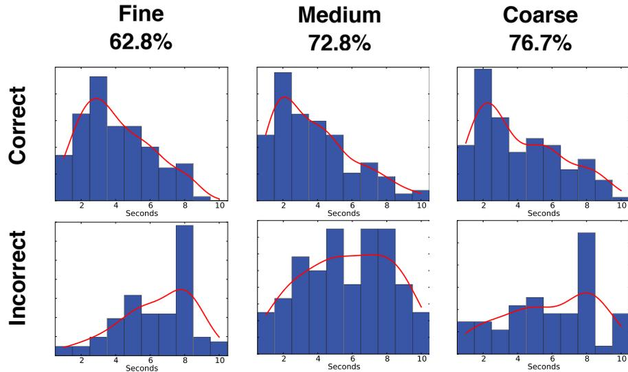
Figure 5.5: The performance of supervoxel semantic retention of actor and action on three levels from the supervoxel segmentation hierarchy: fine, medium and coarse. The percentages on top are computed when both the actor and action of supervoxel perception are correctly matched to ground truth. The middle and bottom rows are the response time figures when the supervoxel perception is correctly matched and incorrectly matched respectively.
