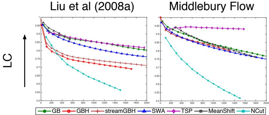
Figure 3.4: Plots for Label Consistency (LC) against the number of supervoxels **per-video** (x-axis). Black arrow indicates the direction of better performance. Plotted dots are the average score of linear-interpolated values from all videos in a dataset at the same number of supervoxels per-video.
