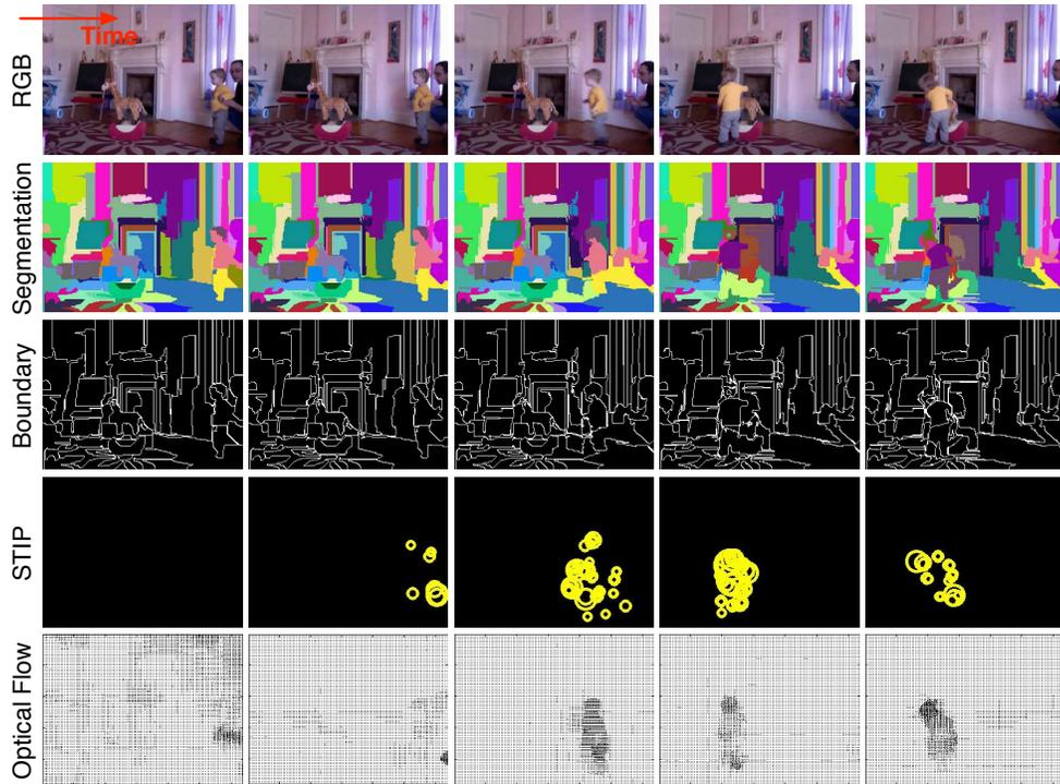
Figure 5.2: A comparison of different video feature representations. From top to bottom rows are: the RGB video, the supervoxel segmentation [221], extracted boundaries of supervoxel segmentation, space-time interest points [98], and optical flow [178].
