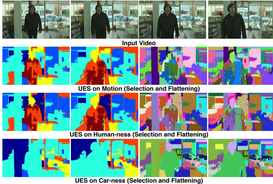
Figure 6.12: UES on Motion, Human-ness and Car-ness on video *nocountryforoldmen* from [65]. For Motion and Human-ness, the moving man is selected from the finer levels, while most others are from coarser levels. For car-ness, the car and nearby regions are selected from finer levels. The red selection around the window is to avoid leaks.
