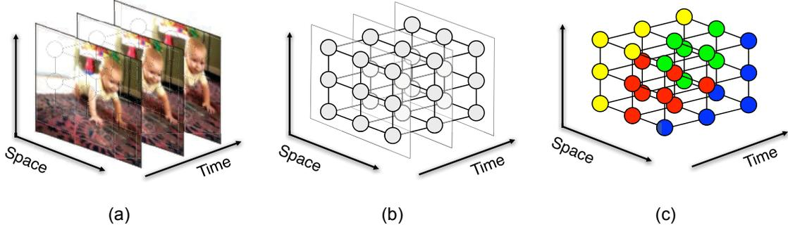
Figure 1.2: Illustration of supervoxel segmentation. (a) A video contains a sequence of frames. (b) A 3D lattice is built with nodes as voxels and edges linking voxels within a frame and across frames. (c) Voxels are being segmented into four groups, i.e. supervoxels, denoted by distinct colors.
