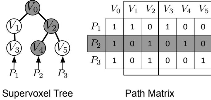
Figure 6.5: Supervoxel tree  $\mathcal{T}$  and the corresponding path matrix  $\mathcal{P}$ . The path  $P_2$  is highlighted to illustrate the path matrix  $\mathcal{P}$  in which each row specifies a root-to-leaf path through the tree.
