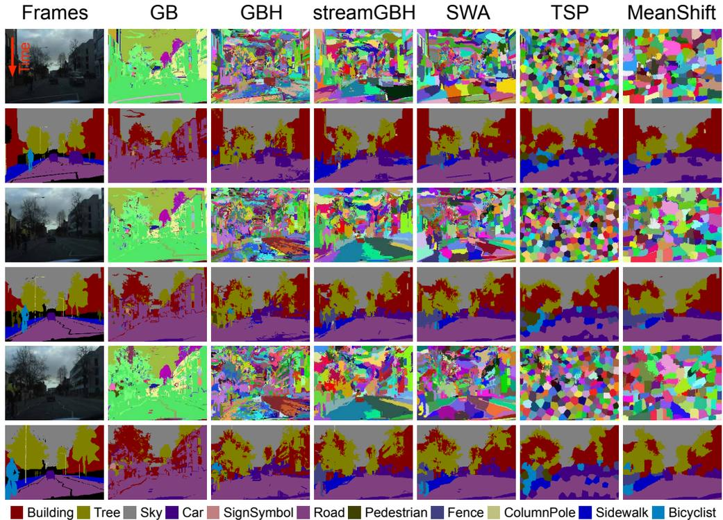
Figure 3.10: Example results on a clip from the CamVid dusk test video. Images in the first column are video frames and groundtruth labels and the remaining columns are individual methods with supervoxel segmentation and semantic labeling on supervoxels.
