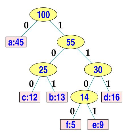
The Huffman coding is a greedy method for obtaining an optimal prefix-free binary code, which uses the following idea: For each i,  $1 \le i \le n$ , create a leaf node  $v_i$  corresponding to  $a_i$  having frequency  $f_i$ . Let  $D = \{v_1, \ldots, v_n\}$ . Repeat the following until  $\|D\| = 1$ .
